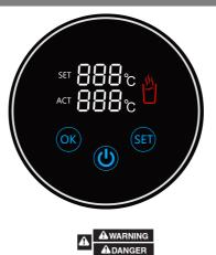
If the electronic instant hot water appliance is empty of water and is turned ON then this will be automatically sensed, the heating element will not energise and the "lack of water" indictor will be flashing on the display panel shown by the flashing of the E3
