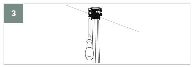
Use a cross screwdriver to tighten the two fixing screws.
