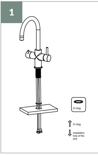
Put the O-ring (B) on the bottom of the tap, then put the four flexible hoses and one silicone tube through the sink hole.
