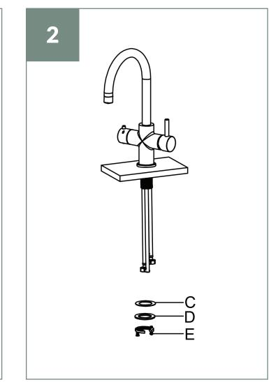
Put the rubber washer (C),metal washer (D), and fixing nut (E) through the hose in turn, fix them on the thread connector, tighten them by hand.
