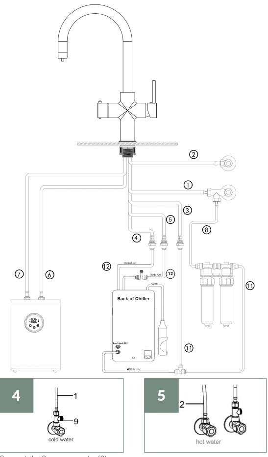
Connect the 3-way connector(9) to the housecold water valve, and connect the hose (1) to the one side of 3-way connector and tighten it with a wrench.
