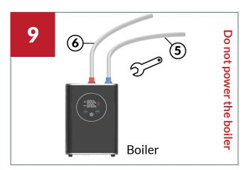
Connect hose (6) to the outlet of the boiler (Red) Please make sure the rubber washer is in place first, hose (5) to the inlet (Blue) and hand tighten them. Using an adjustable spanner tighten further by a maximum of one turn. Do not power the boiler at that stage.
