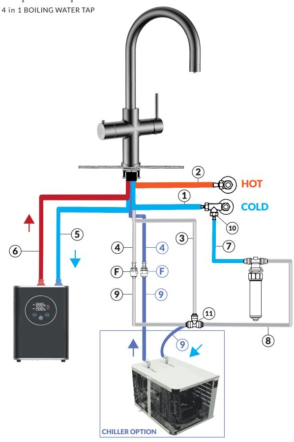
**TOP TIP:** Pass the 3 hoses with nuts through the surface hole first and then pass the 3 hoses without nuts to help with your installation.
