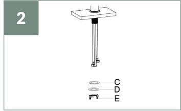
Put the rubber washer (**C**), metal washer (**D**), and fixing nut (**E**) back onto the tap by feeding the hoses through them. Fix them onto the thread at the base of the tap and tighten by hand.
