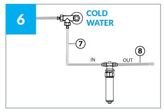
Connect hose (7) to the metal **T piece** on the cold mains and tighten it with an adjustable spanner. Insert the other end of the hose (7) into the filter's inlet. Insert the filter outlet hose (8, plastic 3/8 PE tubing) into the filter's outlet.
