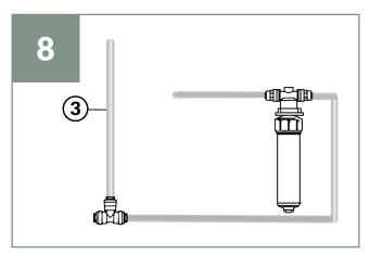
Connect hose (3) to the other side of the **plastic** 3-way connector, by removing the blue clip first and then secure by using the blue clip once attached.
