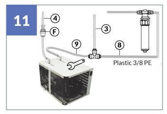
If you are connecting a chiller unit, connect the other end of the **1/4 inch tubing** (**9**) thats connected to (**F**) to the water outlet of the chiller unit. Using another piece of **1/4 inch tubing** (**9**) connect one end to the **plastic 3 way connector** and other to the water inlet on the chiller.
