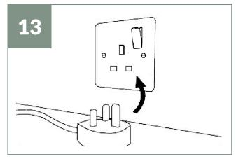
Insert the plugs of the boiler ( and chiller if installed together) into the power socket and **switch on.**
