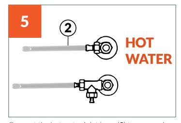
Connect the hot water inlet hose (2) to your mains hot water supply and tighten it with an adjustable spanner.
