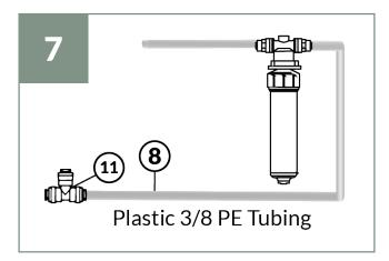
Connect the filter outlet hose (8) to one side of the plastic 3-way connector (11) by removing the blue clip first and then re-attach the clip to secure into place.
