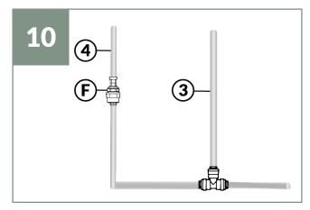
Connect hose (4) to the plastic 1/2" screw to 1/4" push fit connector(F). Insert one end of the 1/4 inch tubing to (F). If you have a chiller now go to step 11. Otherwise, connect the other end of the 1/4 inch tube (9) to the plastic 3 way connector and move to step 12.
