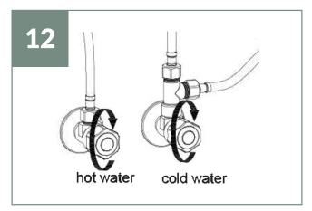
Turn on your mains hot and cold water, check and ensure no connections are leaking. Turn the handle for boiling water to fill the boiler. No water will come out of the tap until the boiler is full.
