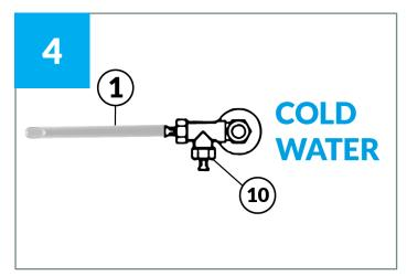
Connect the metal T piece (**10**) to your mains cold water supply. Then Connect the cold water inlet hose (**1**) to one side of the **T piece** and tighten it with an adjustable spanner.
