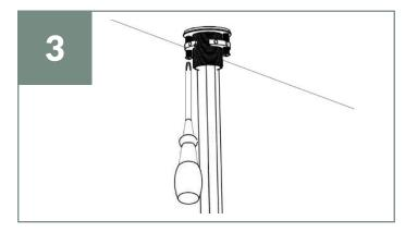
Use a philips screwdriver to tighten the two fixing screws.
