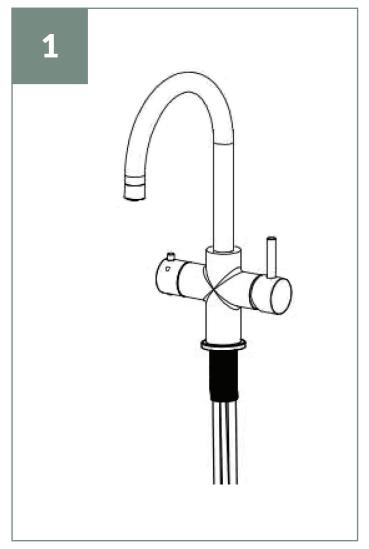
Remove the rubber washer (**C**), metal washer (**D**), and fixing nut (**E**) from the base of the tap. Then put all the flexible hoses through the tap hole.
